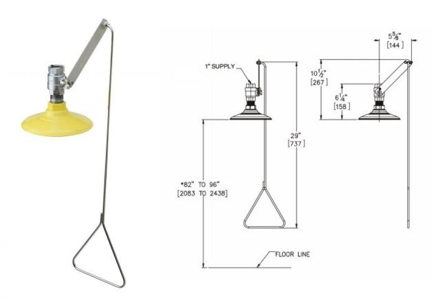
Model S1100 is our vertical ceiling mounted safety shower with plastic head. Complete with plastic shower head, stainless steel pull handle and supplied with 1" chrome plated brass stay open ball valve.
